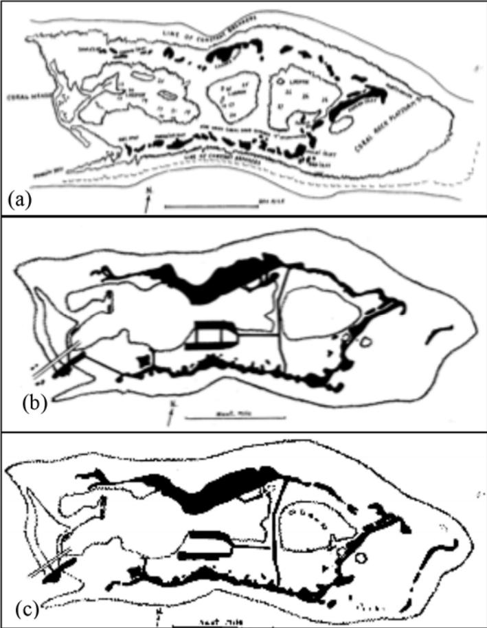
Figure 1: Changes at Palmyra over time: (a) the atoll in 1913, with open lagoon and many hoa, (b) in 1944, after the Navy's construction, including a road connecting the motu and causeway bisecting the lagoon, and (c) in 1958 after a decade of erosion. (Dawson, 1958)
