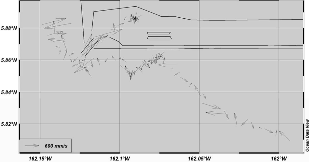
Figure 13: Surface current profile from Acoustic Doppler Current Profiler at Palmyra Atoll (with rough sketch of Palmyra for scale). Recorded May 27, 2007.
